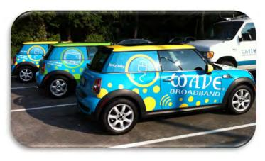
installers applied the wrap to one of the MINI Coopers and once everyone at Wave Broadband saw the finished product, they were sold. The team had the green light to move forward with wrapping the other five vehicles. To complete the wraps, FASTSIGNS used solvent prints on 3M IJ-180c vinyl with 3M Window Perf.
