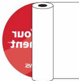
LAMINATE IMAGE WITH WHITE VINYL THAT HAS A CLEAR ADHESIVE
